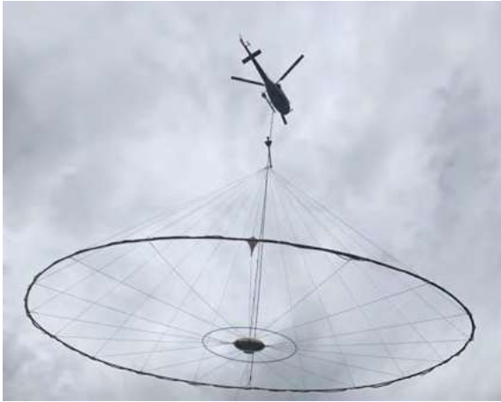
Figure 1. HoriZOND AEM system.
