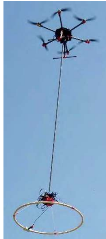
Figure 4. The UAV-mounted PDI-50 TDEM receiver.
